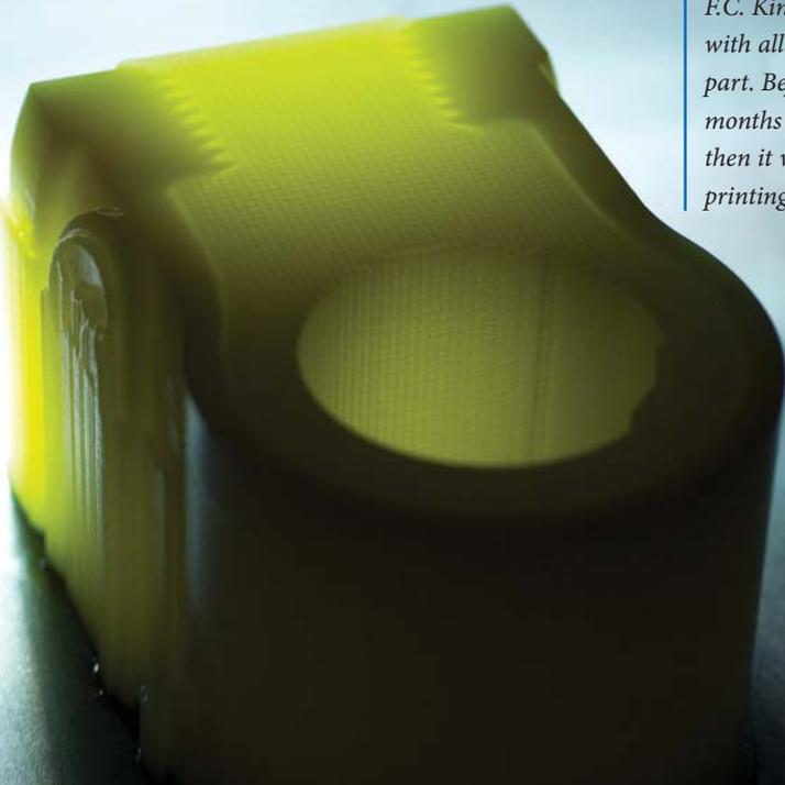
*F.C. Kingston's side outlet PRV is printed with all the threads to simulate the completed part. Before 3D printing, it could take several months to get the part from suppliers and then it would need to be machined. 3D printing eliminates those steps.*
