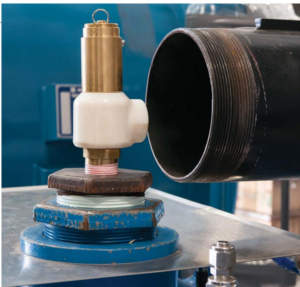
*Above: F.C. Kingston's side outlet PRV is successfully air-tested at the National Board lab.
