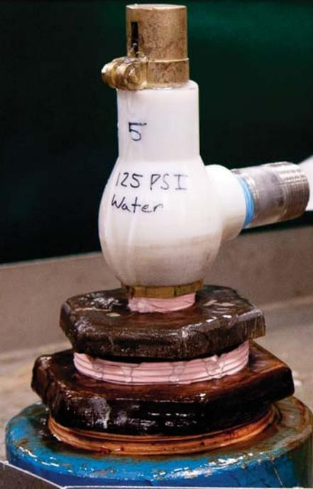
*The National Board Test Lab's very first 3D printed valve part from F.C. Kingston, a liquid service PRV, undergoes successful water testing.*
